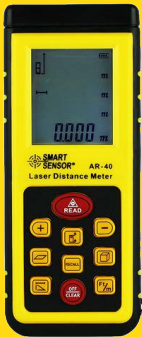
Laser Distance Meter AR40 0.3~40m
