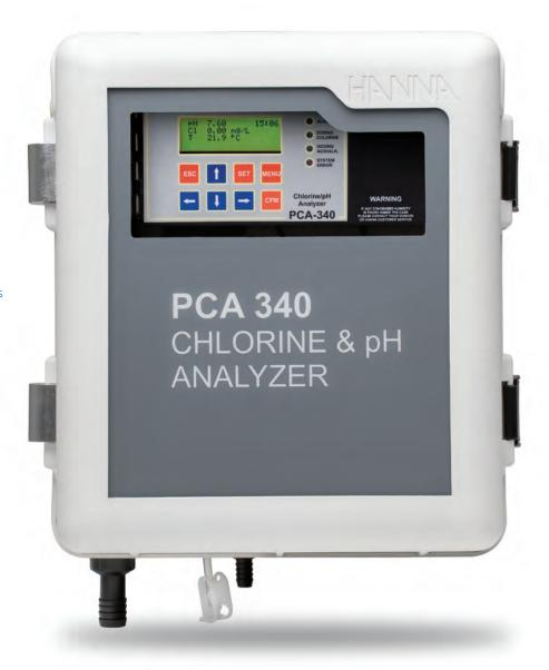
The PCA family are process analyzers for the continuous measurement of chlorine, pH (PCA320, PCA330, PCA340) and temperature. These analyzers feature built in data logging, RS485 digital output, dosing relays, and alarm relays packaged in a wall mount Nema 4x enclosure. The PCA340 also features two analog outputs.
