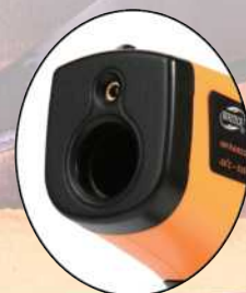
Temperature sensor and positioning laser
