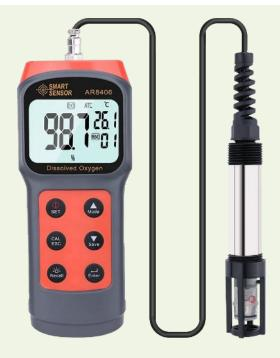
Measuring dissolved oxygen is important in many applications because it is an indicator of the health of an aquatic ecosystem. Low levels of dissolved oxygen can be harmful to fish and other aquatic organisms, and high levels of dissolved oxygen can indicate the presence of pollutants or other environmental disturbances.
