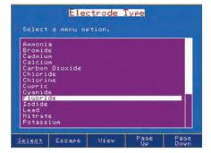
Selectable ISEs preprogrammed with molecular weight and ion charge
